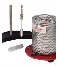
Option: Disposable Sample Chamber with Optional Disposable Spindle SC4-27D\* is ideal for asphalts or any difficult-to-clean material.
