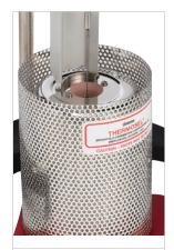
Alignment Bracket ensures concentricity of spindle and sample chamber.
