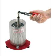
**Extracting Tool enables** the sample chamber to be handled easily and safely.
